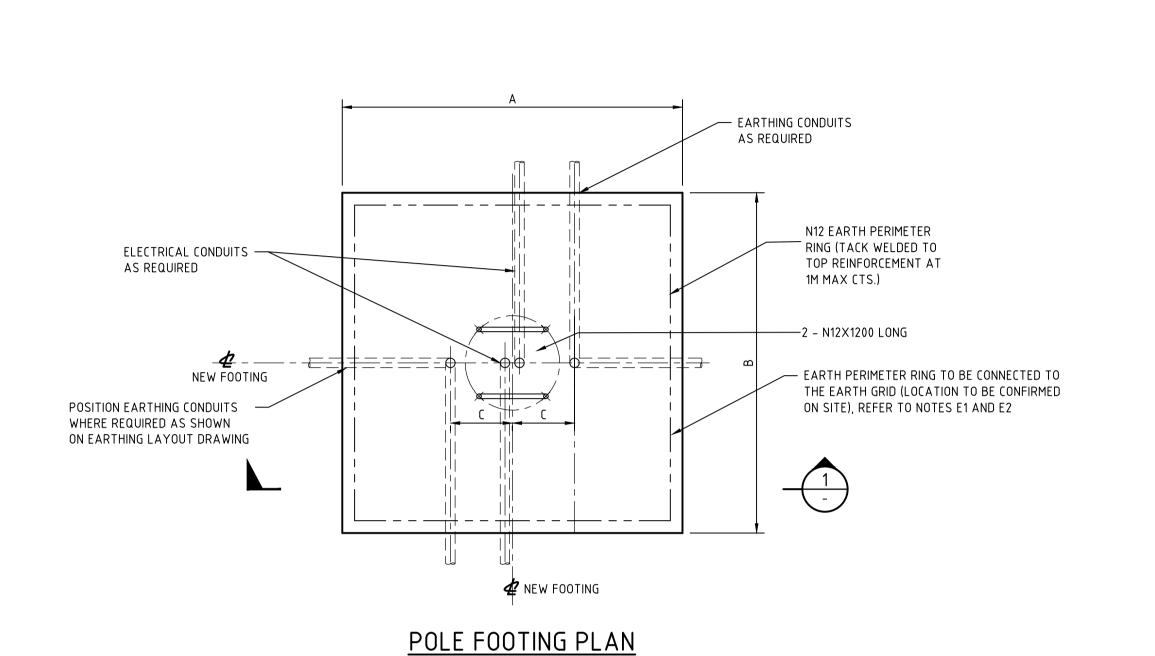
FOR LOCATION OF FOOTINGS REFER TO SITE SPECIFIC FOOTING PLAN. REFER TO APPROPRIATE LAYOUT OF PITS & DUCTS DRAWING FOR DIRECTION OF CONDUITS
