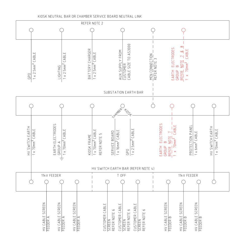
COMBINED EARTHING CONFIGURATION FOR ADJACENT CHAMBER SUBSTATIONS WITH SHARED ELECTRODE GROUPS
