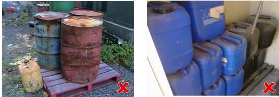
Drums in poor condition, not banded, labelled or covered can leak and contaminate land or waterways
