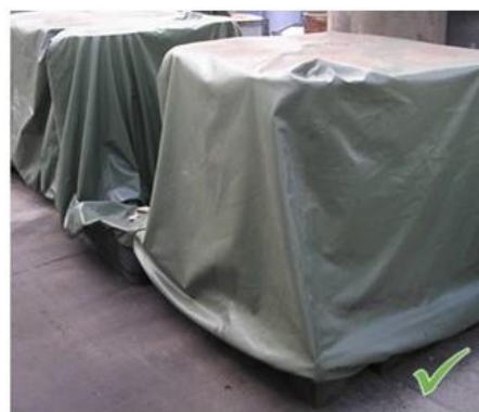
Bunded pallets should be covered when exposed to the weather
