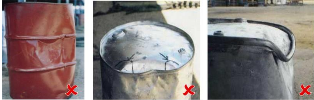
Sharp indents and damage to the rolling hoops or edges are potential leak points
