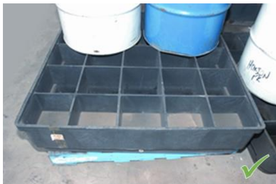
Bunded pallets can be used for temporary storage of drums
