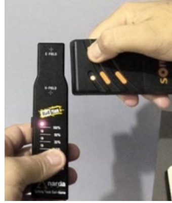
The RF EME meter is calibrated to the general public limit
