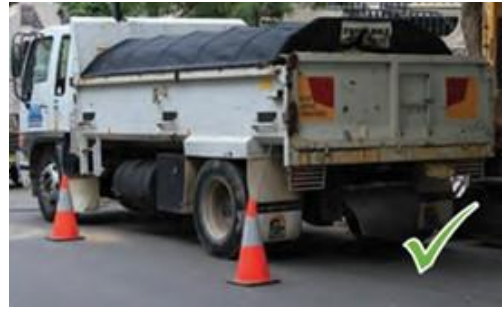
Cover loads to prevent pollution
