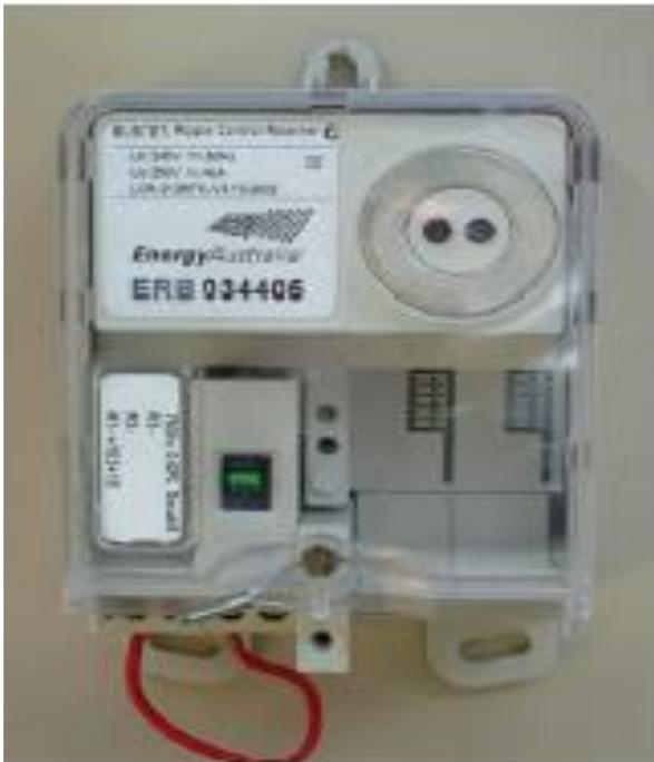
Figure A3: Ripple Receiver
