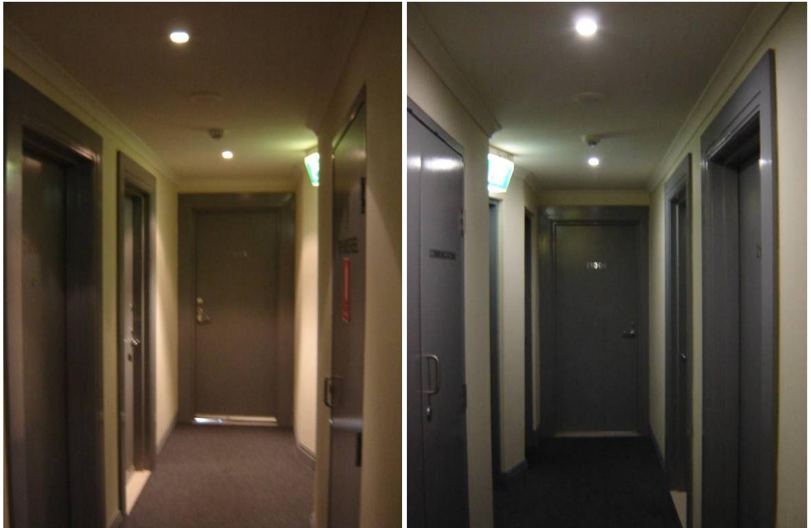
As shown in the photos above, the light distribution of the tungsten halogen downlights is much more focused in the downward direction while the compact reflectors have a comparatively wide angle of light distribution. This study found that the uniformity of illuminance provided by the tungsten halogens is below the level recommended by the Australian Standards.
