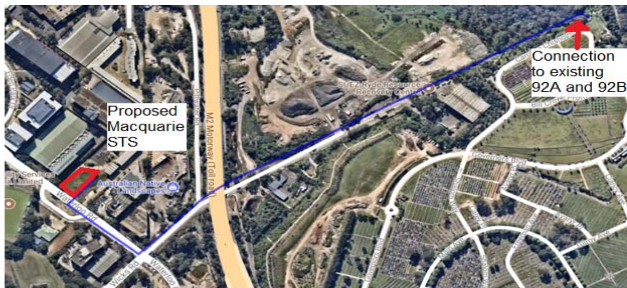
Figure 6-1 - Proposed new STS site and route plan for the new 132kV feeder
