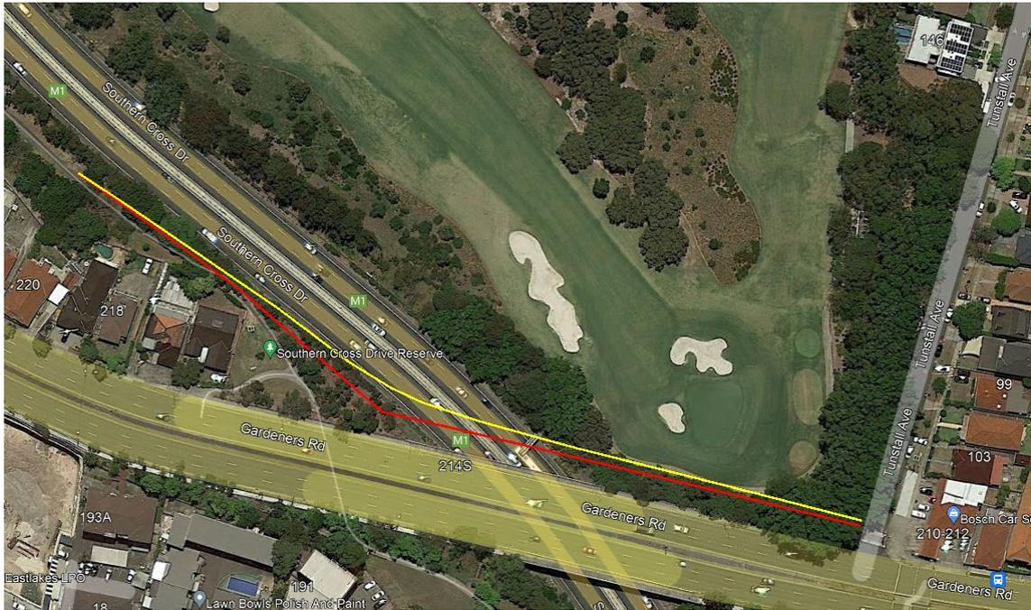
Figure 1-3 Horizontal Directional Drilling locations adjacent to Southern Cross Drive. Option 1 in Red and Option 2 in Yellow.
