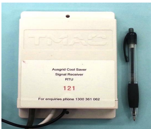
Figure 3: Demand response enabling device/ Signal receiver (3G model used for Phase 3 of the trial)
